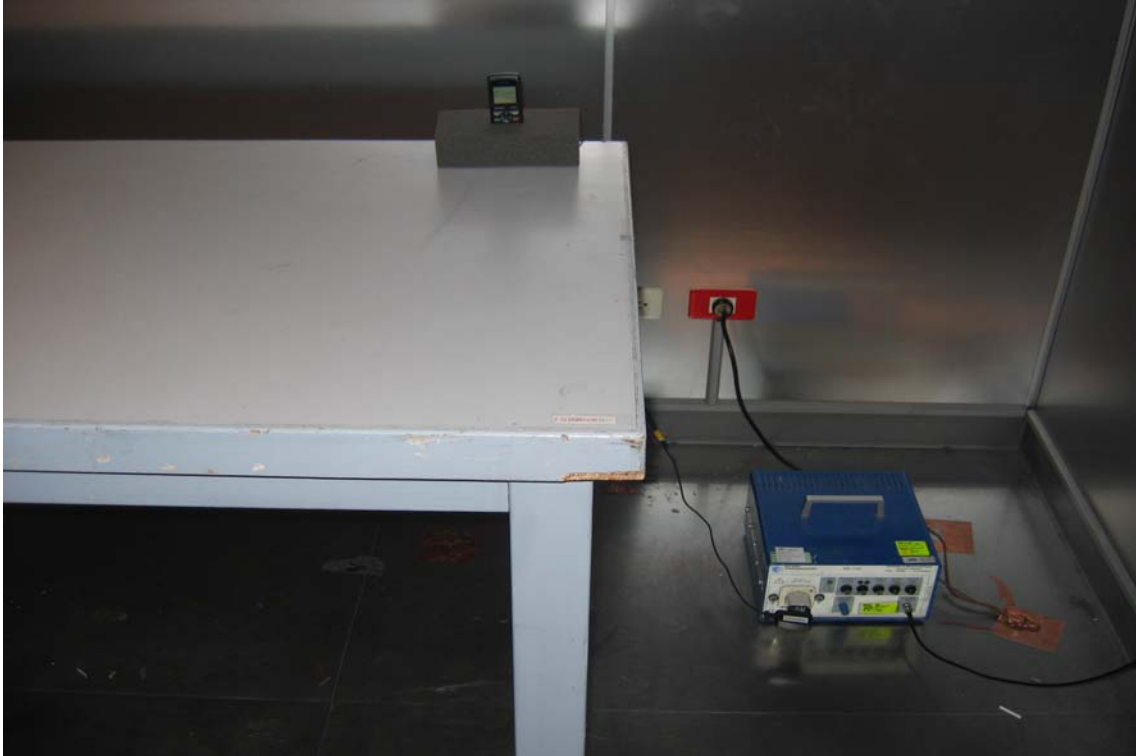
Conducted Emission Test Setup Photo(Power Adaptor)
