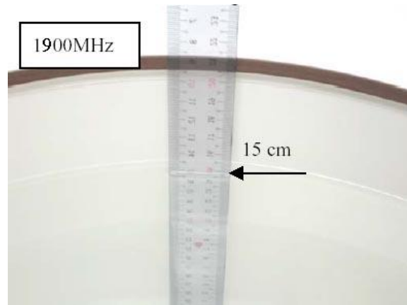
Fig.5 Photograph of the Tissue Simulant Fluid Liquid depth 15cm for Body-Worn
