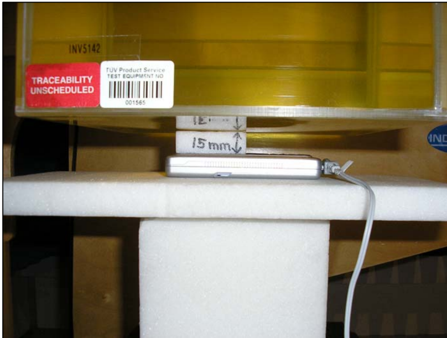
Figure 31: Positional Photograph of the Sagem A2005sca+ Handset Front Facing Phantom 15mm from the Phantom with Simple Hands Free Accessory (SAR Body Test)
