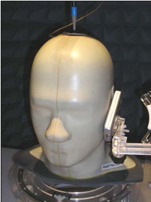
Figure 27: Positional Photograph of the Sagem A2005sca+ Handset in LH Cheek Position (SAR Head Test)
