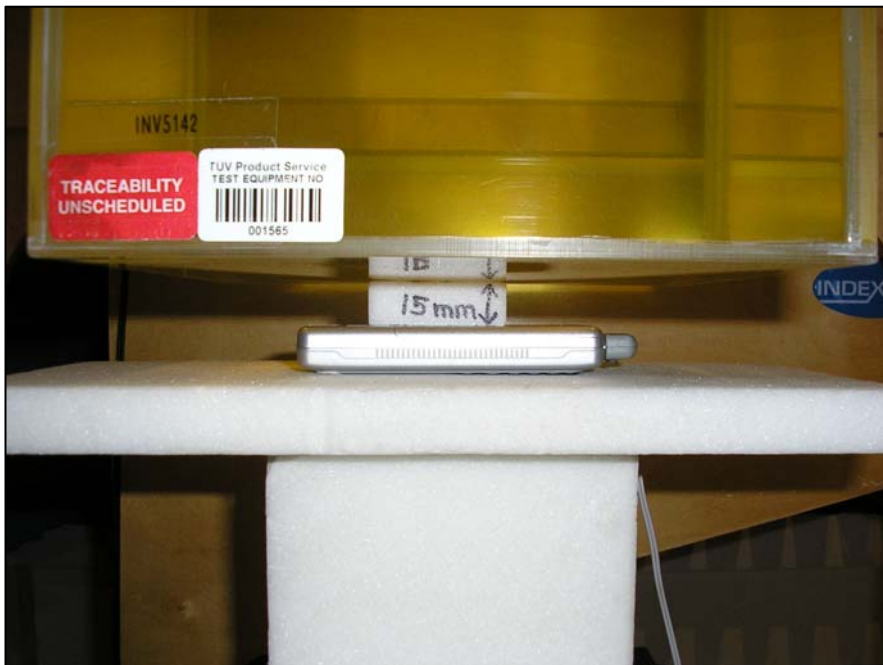
Figure 32: Positional Photograph of the Sagem A2005sca+ Handset Rear Facing Phantom 15mm from the Phantom with Simple Hands Free Accessory (SAR Body Test)
