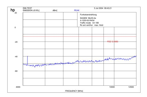
f < 1 GHz : RBW/VBW: 100 kHz Carrier suppressed with a rejection filter f ≥ 1GHz : RBW/VBW 1 MHz
