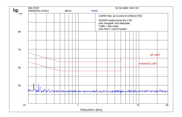
We used 100 kHz for RBW/VBW Peak, 9 kHz for CISPR QP measurement.
