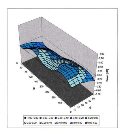
Spherical Isotropy Error < ± 0.4 dB
