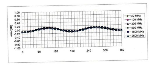
Axial Isotropy Error < ± 0.2 dB
