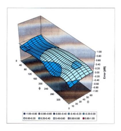
Spherical Isotropy Error < ± 0.4 dB
