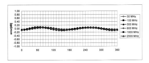
Axial Isotropy Error < ± 0.2 dB
