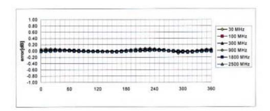
Axial Isotropy Error < ± 0.2 dB
