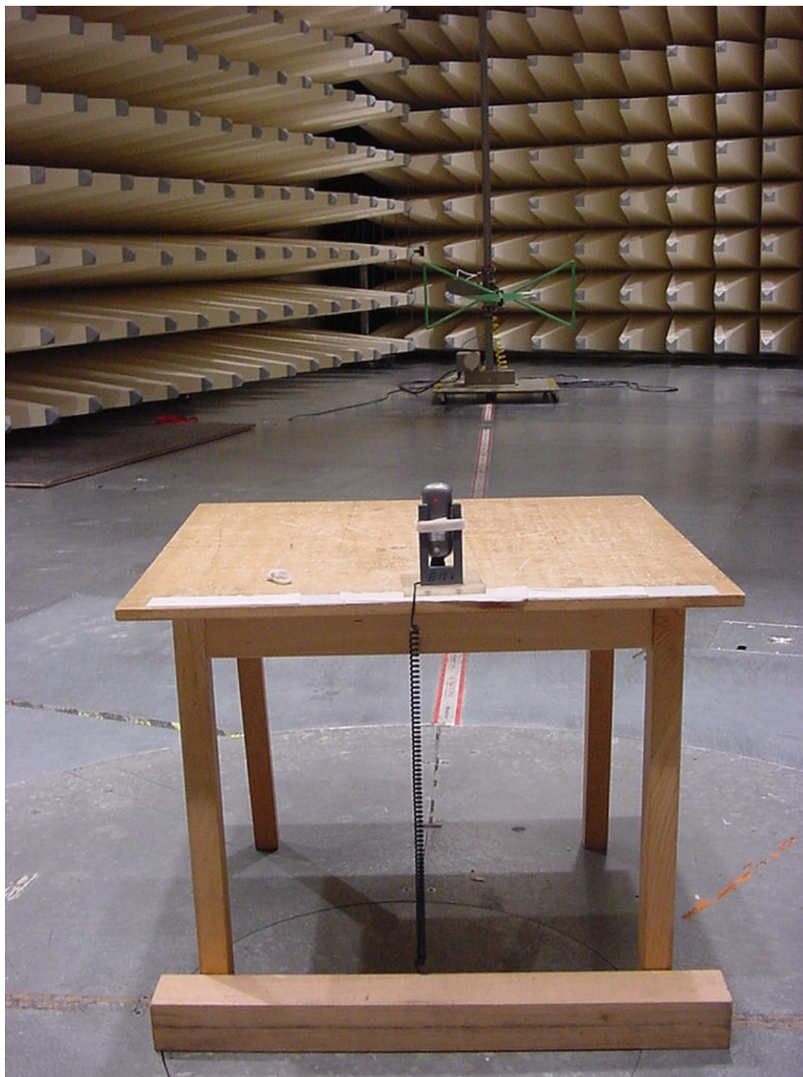
Photo 3 (Radiated Emissions): Cigar Light Adapter
