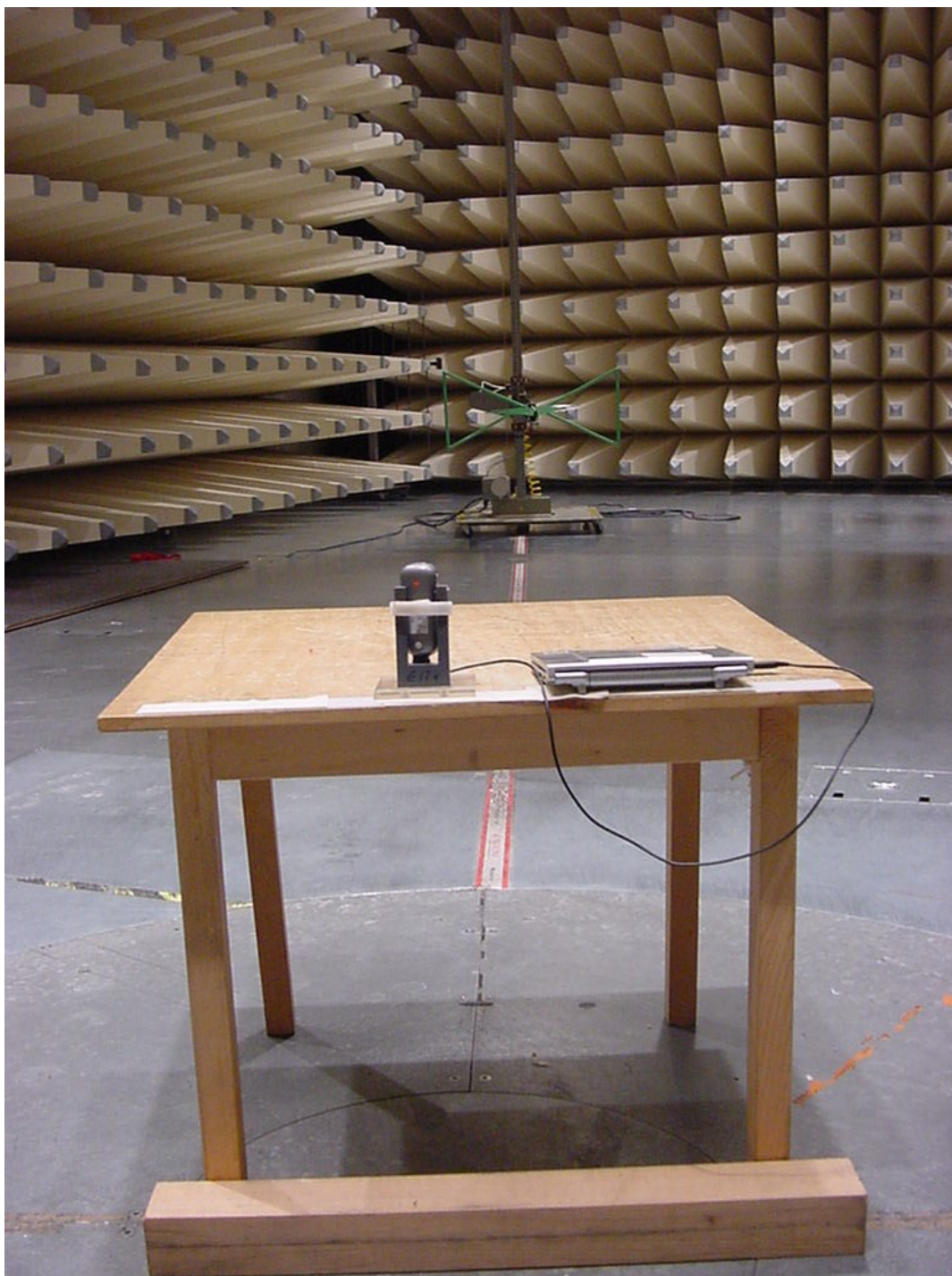
Photo 4 (Radiated Emissions): USB Cable
