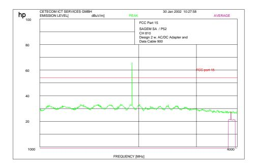
Peak at 1909.8 MHz shows the carrier frequency suppressed by narrow band rejection filter
