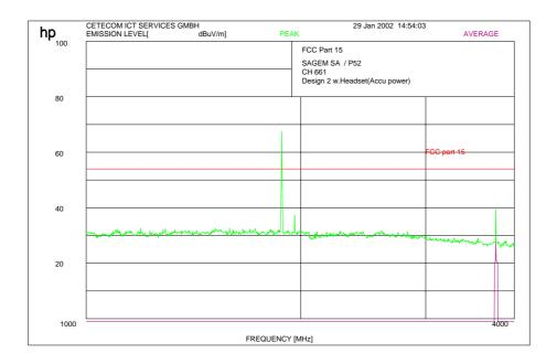
Peak at 1880.0 MHz shows the carrier frequency suppressed by narrow band rejection filter
