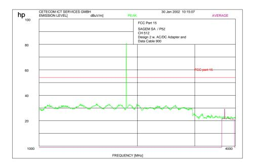
Peak at 1850.2 MHz shows the carrier frequency suppressed by narrow band rejection filter
