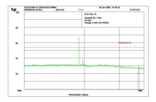
Peak at 1880.0 MHz shows the carrier frequency suppressed by narrow band rejection filter
