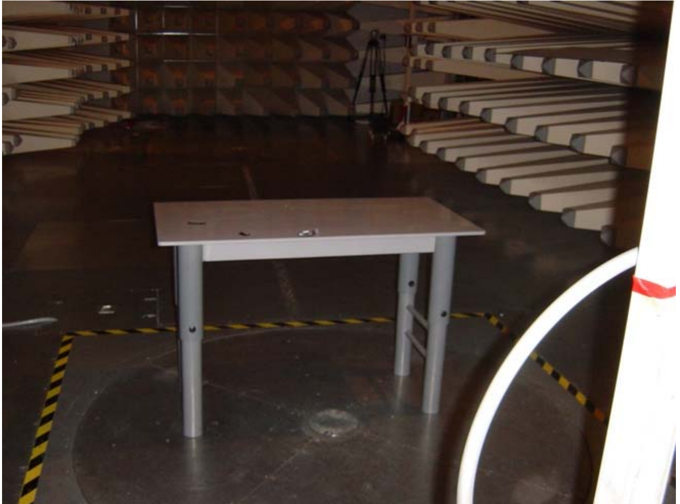
Set-up for Radiation Emission (Transceiver)
