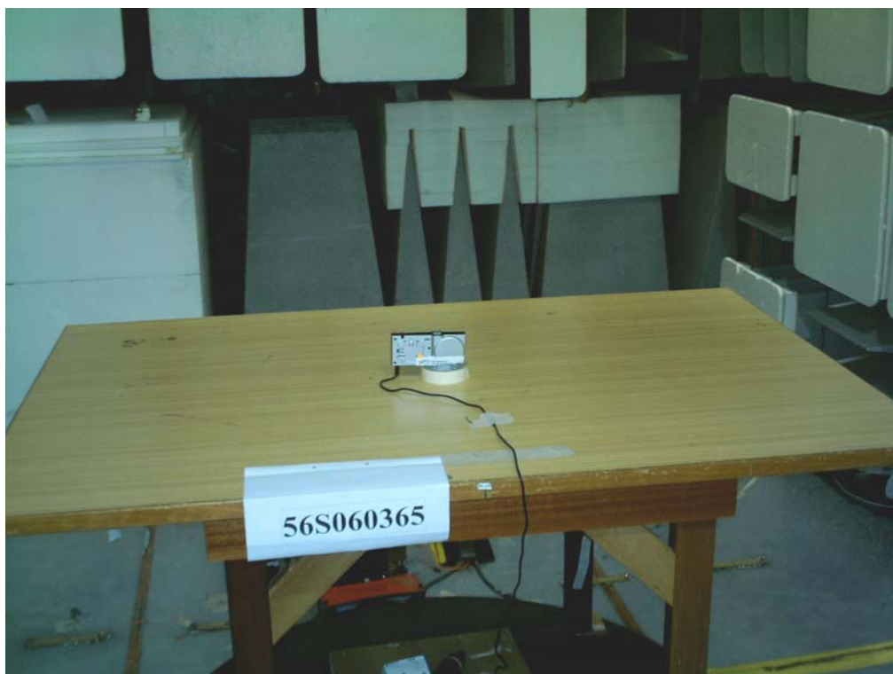
Radiated Emissions Test Setup (Rear View)
