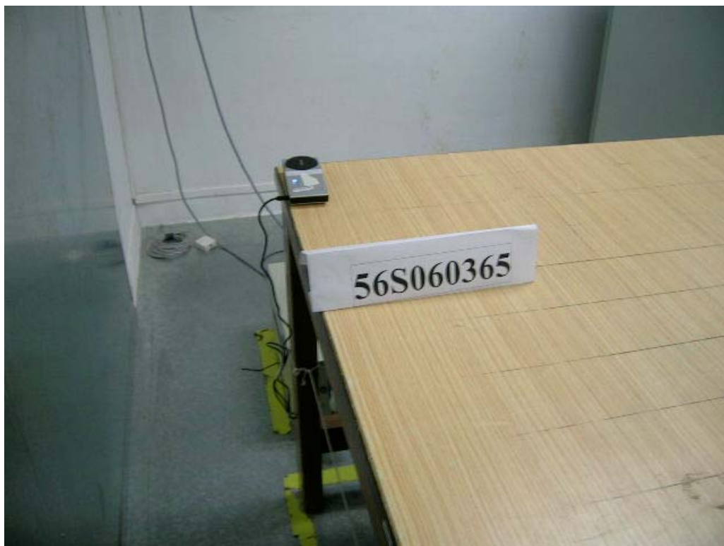
Conducted Emissions Test Setup (Rear View)
