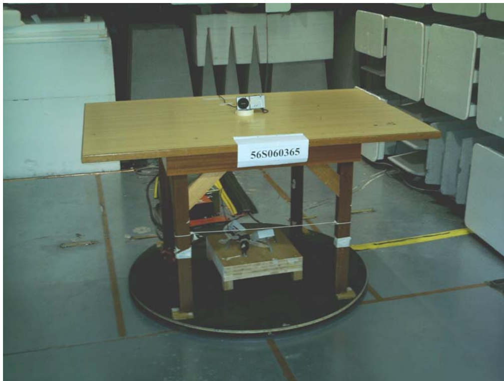
Radiated Emissions Test Setup (Front View)
