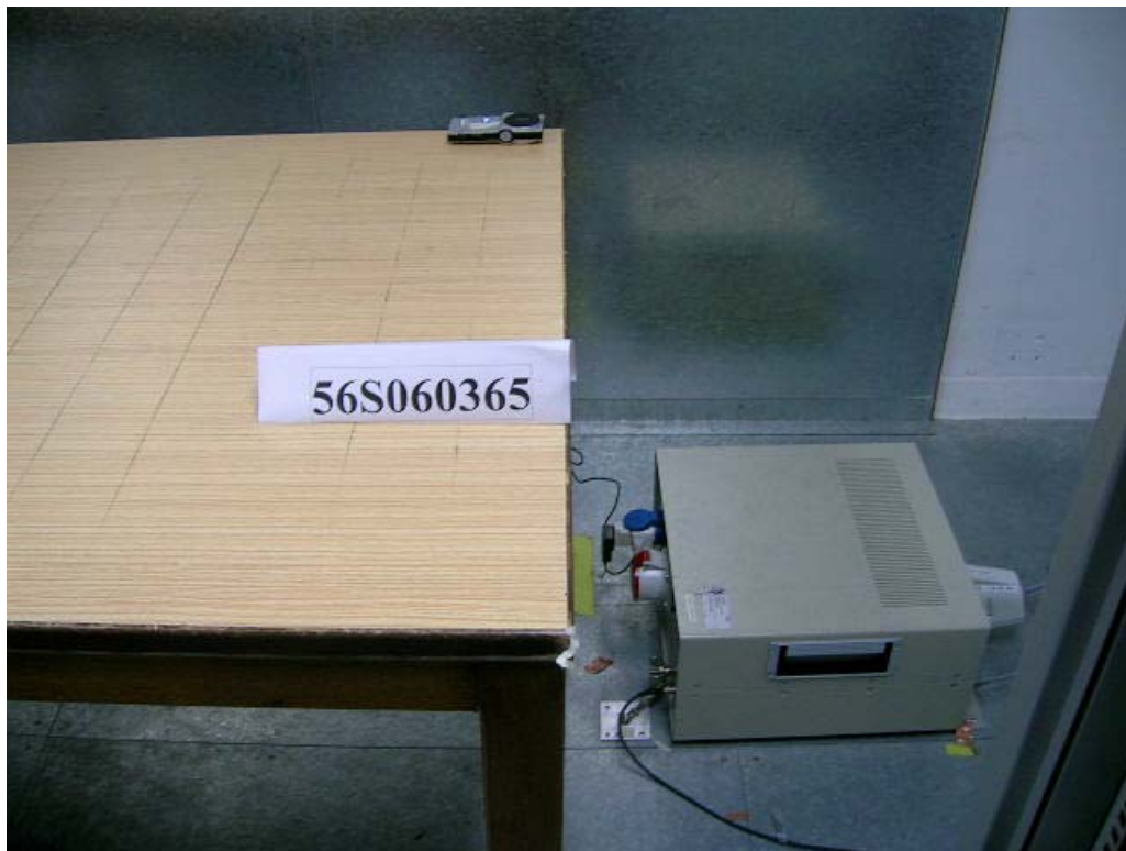
Conducted Emissions Test Setup (Front View)
