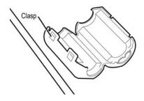
Position the ferrite bead on the cable as close as possible to (but not inside) the MorphoAccess.
