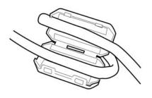
4. Close the two halves of the ferrite bead and securely fasten the clasps without pinching the cables.
