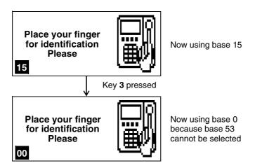
If the identification is successful, the terminal triggers the access or returns the corresponding ID to central security controller.
