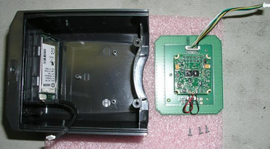
MA110 HID reader disassembled from top assembly
