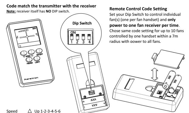
To start the fan press speed button To change speed of fan press  $\triangle$  or  $\nabla$  (indicated by a short buzzer sound) LCD indicates maximal speed (max)
