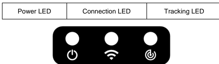
The following table gives the standard configuration of the status LEDs. The specific response can be modified via the application software.
