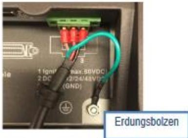
The other end of the yellow-green power supply cable must be connected to the vehicle's chassis. Connect the power supply cable of the ZenoCCU as directly as possible to the battery and not to power supply lines with a great deal of interference (e.g. the engine power supply) or otherwise affected by consumers. Connecting the ZenoCCU to large electrical loads, such as converters for the forklift motor may result in random restarts, malfunctions and/or irreparable damage to the device.
