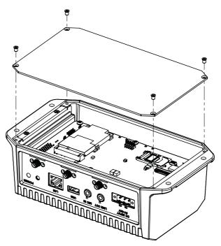
Figure 3.1 Install peripheral in the system
