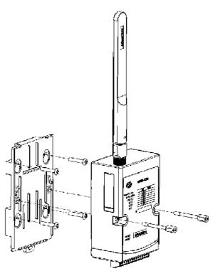
Figure 3.6 Wall Mounting Install 1
