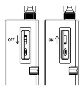
Figure 1.7 WISE-4210 Battery Switch
