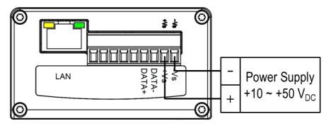
Figure 3.10 WISE-4210-AP Power Wiring
