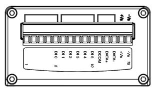
Figure 2.5 WISE-4210-S251 Pin Assignment
