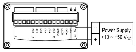
Figure 3.12 WISE-4210-S251 Power Wiring
