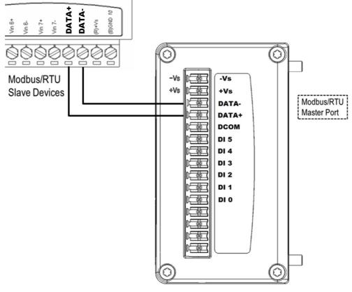
Figure 2.8 WISE-4210-S251 RS-485 Wiring Diagram
