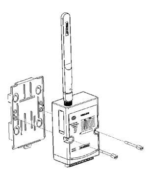
Figure 3.3 DIN Mounting Install
