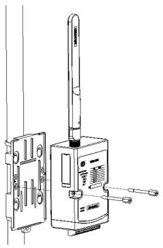
**Figure 3.9 Pole Mounting Back**
