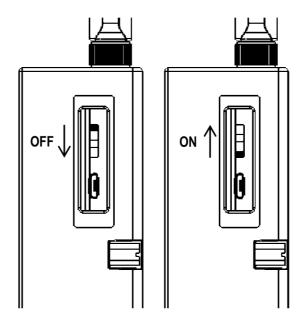
Figure 3.14 WISE-4210 Battery Switch
