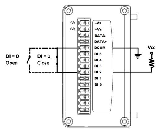
Figure 2.7 WISE-4210-S251 Digital Input Wiring Diagram
