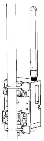
**Figure 3.8 Pole Mounting Front**
