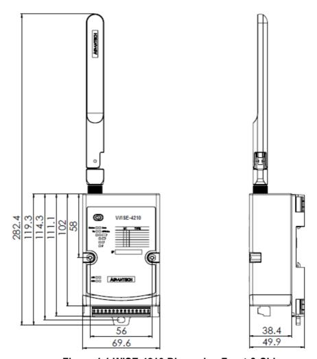
Figure 1.1 WISE-4210 Dimension Front & Side
