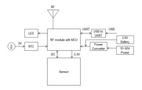
Figure 2.4 WISE-4210-S231 Block Diagram
