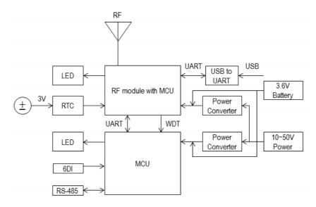
Figure 2.6 WISE-4210-S251 Block Diagram
