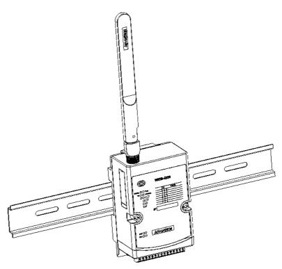
Figure 3.4 DIN Mounting Front
