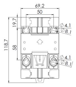
Figure 3.2 WISE-4000 Series Mounting Kit Dimensions
