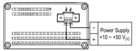
Figure 3.11 WISE-4210-S231 Power Wiring
