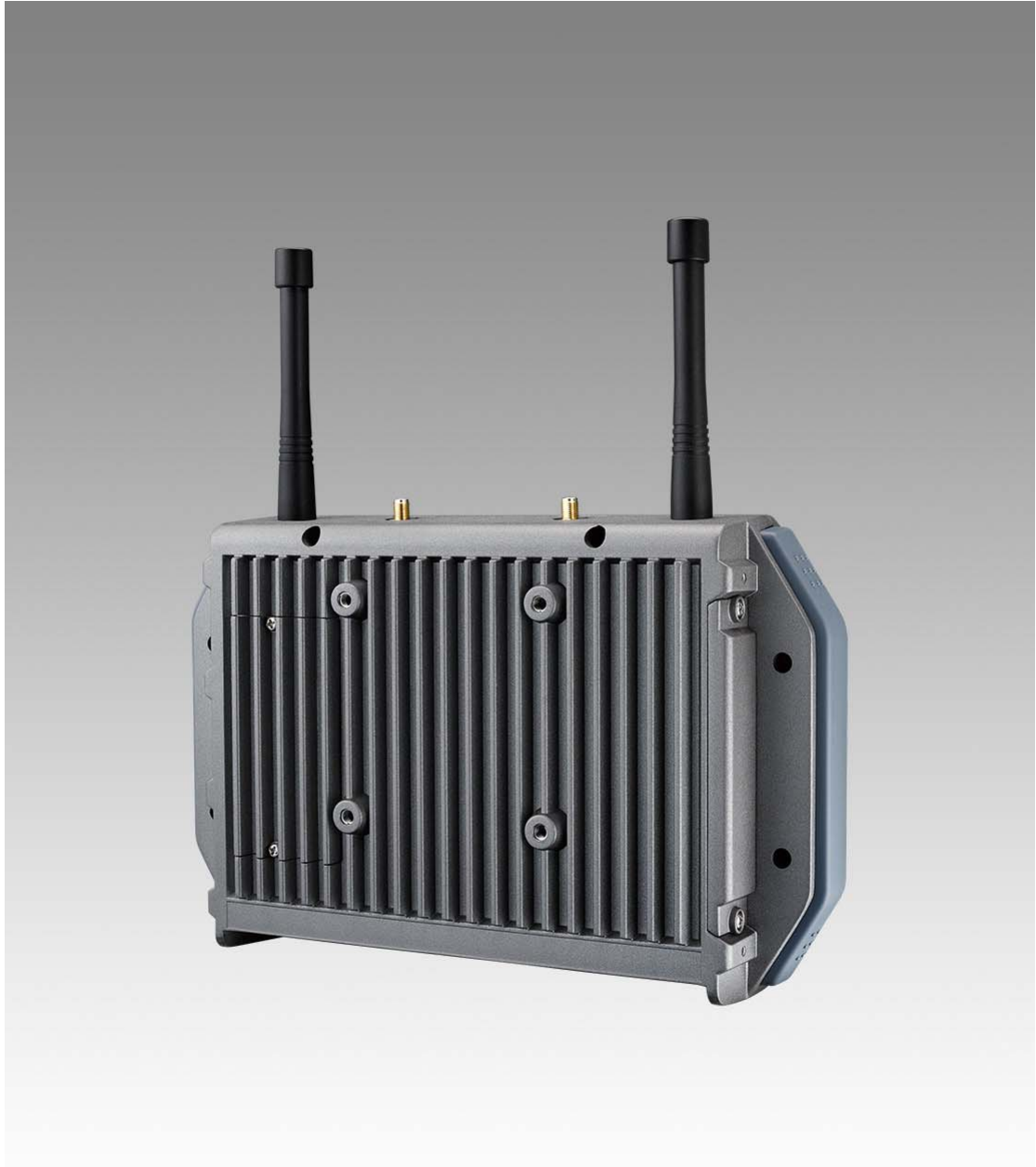
Figure 2.3 Side View of TREK-773
