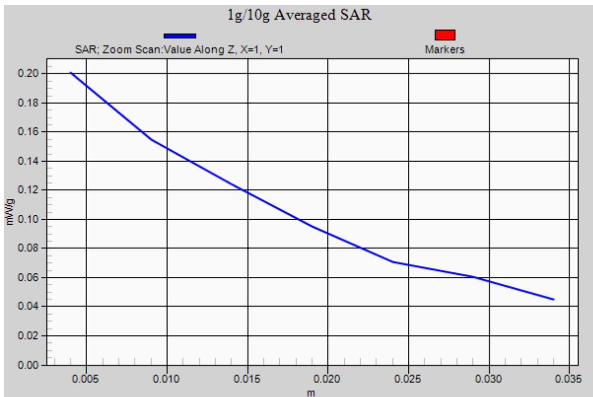
**#21 GSM850\_GPRS10\_Bottom\_0cm\_Ch251\_Main\_Battery2****DUT: 141109**
