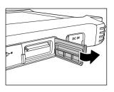
2. Press the SD card inwards to eject it from the slot.
