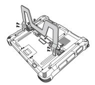
3. Pull to adjust the stand to desirable angle.
