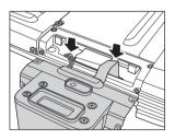
5. Screw to secure the scanner module onto the tablet PC.
