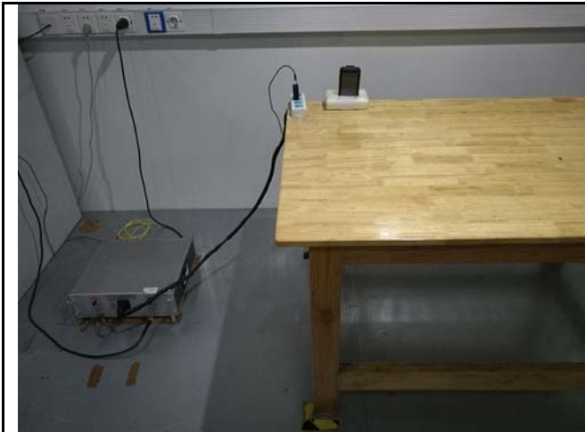
Conducted Emissions Test Setup Front View
