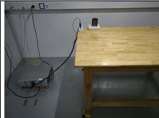
Conducted Emissions Test Setup Front View
