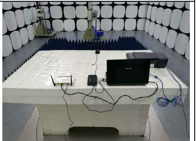
Radiated Emissions Test Setup Above 1GHz
