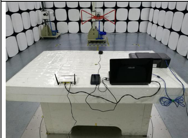
Radiated Emissions Test Setup Below 1GHz
