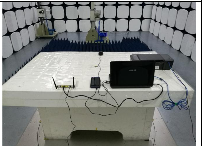
Radiated Emissions Test Setup Above 1GHz
