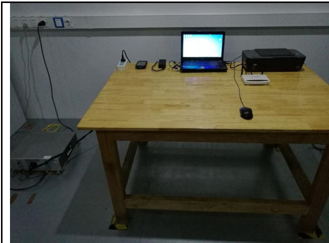
Conducted Emissions Test Setup – Front View
