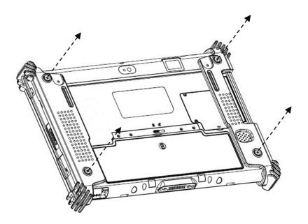
2. Remove the rubber bumpers on the left and right.
