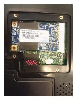
2. Unscrew and remove SSD from the slot.
