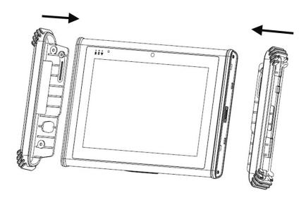
3. Screw the rubber bumpers on left and right properly into the MIT-W101.
