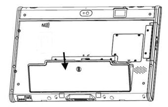
2. Lock to secure the battery once it is properly to be inserted.
