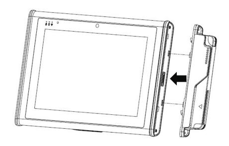
3. Screw to secure the expansion module onto the MIT-W101.
