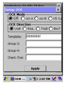
The imager is able to read machine readable fonts used in optical character recognition (OCR). The imager can read from 6 to 60 point OCR type-face.
