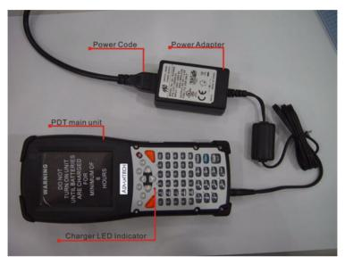
When charging the battery pack, the charge indicator on the PDT turns Red. After the battery pack is fully charged, the indicator turns Green.
