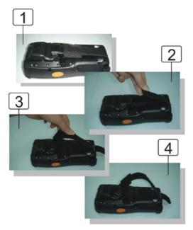
2. Turn the locking screws (right and left) downwards and lift the battery cover away from the PDT.
