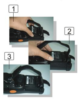
4. Replace the battery cover by inserting the top first, and then press the bottom in firmly. Turn the locking screws (right and left) upwards to secure the cover to the PDT.
