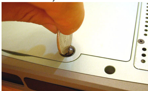
Figure 2.11 Replacing the screws
