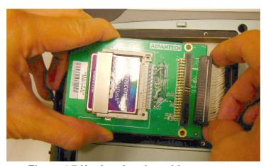
Figure 4.7 Unplugging the cable connector
