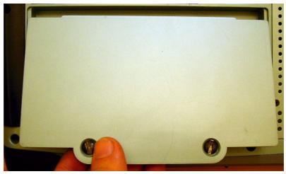
Figure 4.1 Removing the battery pack
