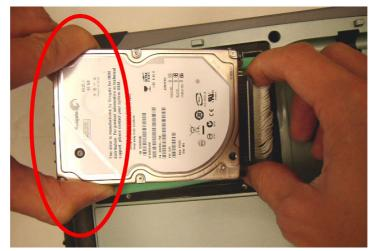
Figure 4.5 Correct Removal of the HDD
