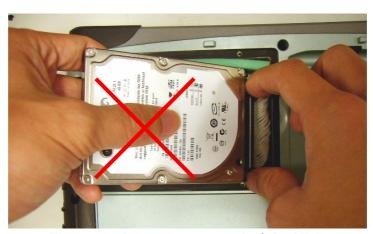
Figure 4.6 Incorrect removal of the HDD
