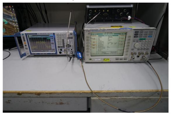
Radiated Emission Set up Photos For Band 5, Band 25 Below 1GHz
