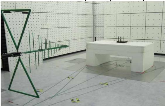
Radiated Emission Set up Photos (Above 1GHz)
