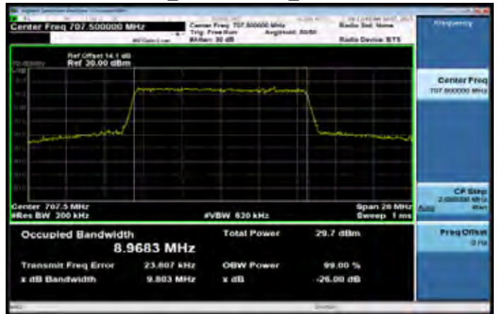
Band12 10MHz_16-QAM 50 0_MidCH23095-707.5
