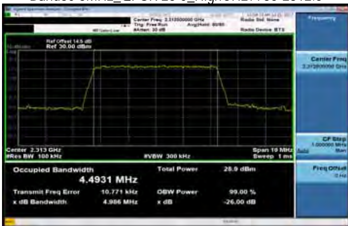
Band30 5MHz_QPSK 25 0_HighCH27735-2312.5
