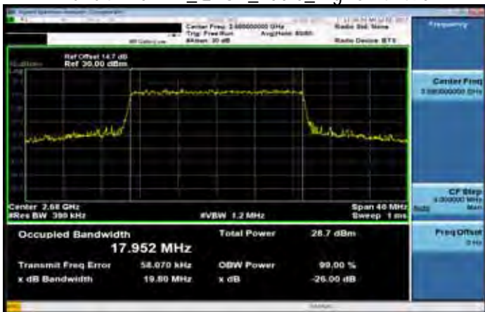
Band41 20MHz_QPSK_100 0_HighCH41490
