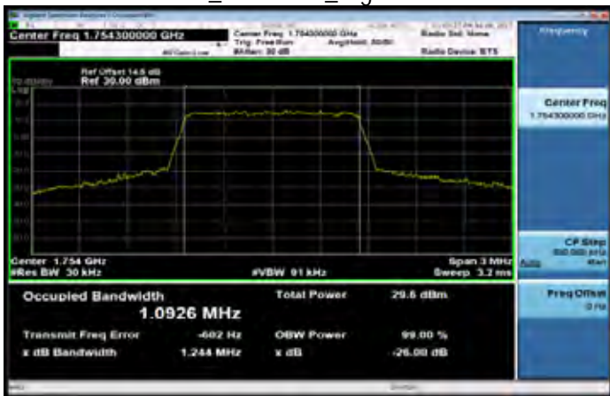
Band4 1.4MHz_QPSK 6 0_HighCH20393-1754.3
