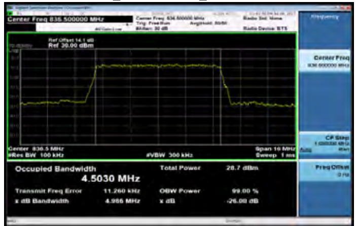
Band5 5MHz_16-QAM 25 0_MidCH20525-836.5
