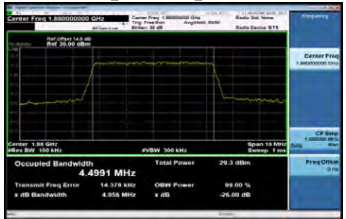
Band2 5MHz_16-QAM 25 0_MidCH18900-1880
