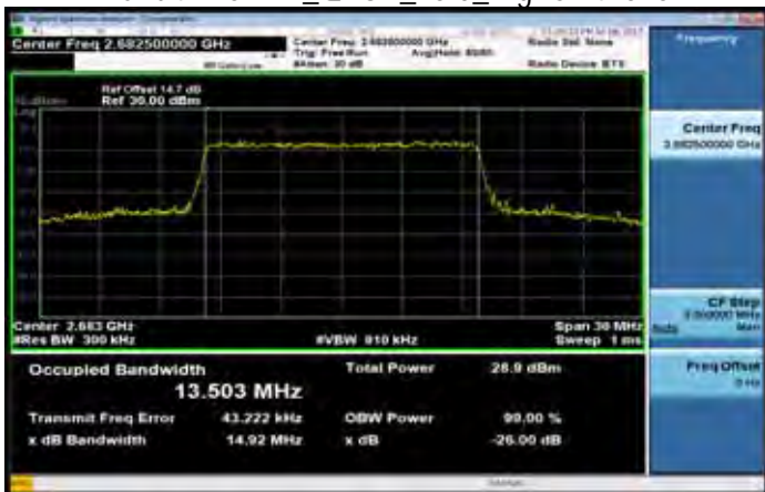
Band41 15MHz_QPSK_75 0_HighCH41515
