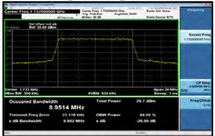
Band4 10MHz_16-QAM 50 0_MidCH20175-1732.5
