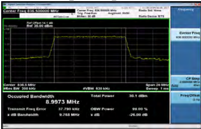
Band5 10MHz_QPSK 50_0_MidCH20525-836.5
