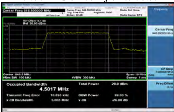
Band5 5MHz_QPSK 25 0_HighCH20625-846.5
