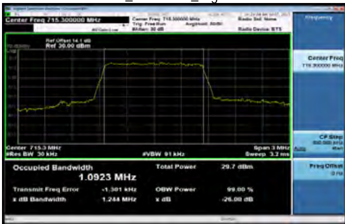
Band12 1.4MHz_QPSK 6 0_HighCH23173-715.3
