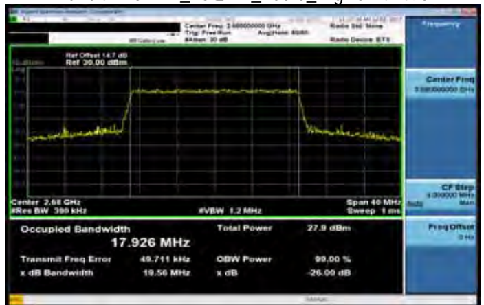
Band41 20MHz_16QAM_100 0_HighCH41490
