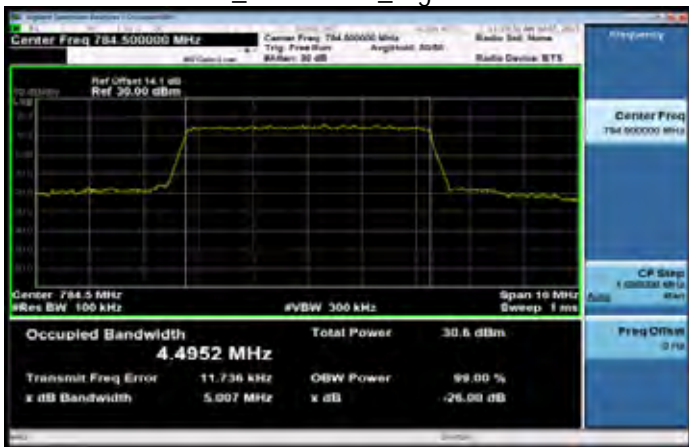
Band13 5MHz_QPSK 25 0_HighCH23255-784.5
