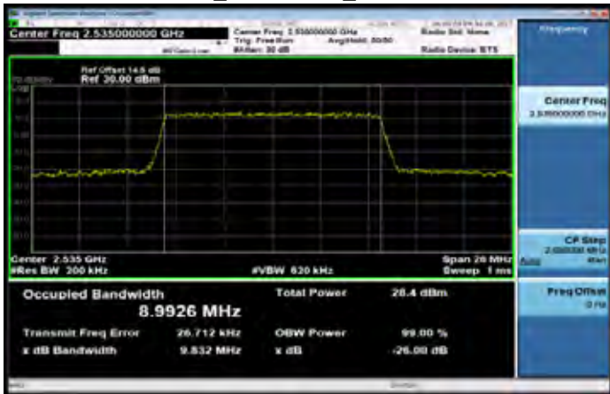
Band7 10MHz_QPSK 50_0_MidCH21100-2535
