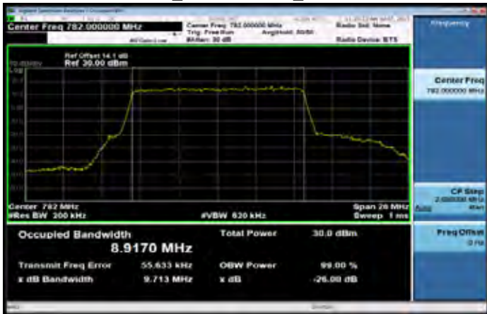
Band13 10MHz_16-QAM 50 0_MidCH23230-782
