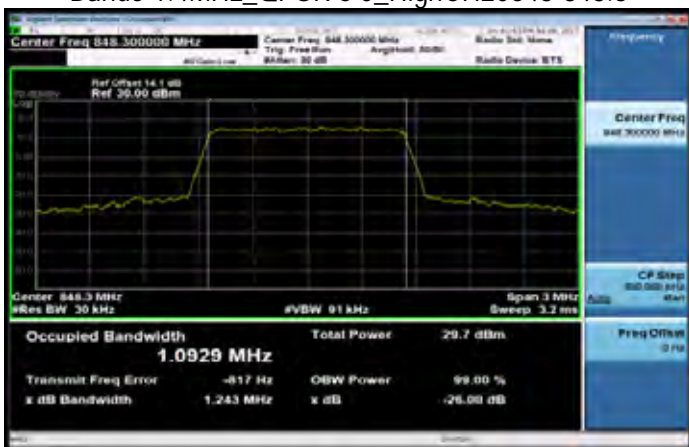
Band5 1.4MHz_QPSK 6 0_HighCH20643-848.3
