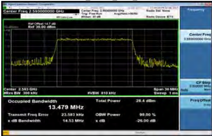
Band41 15MHz_QPSK_75 0_MidCH40620
