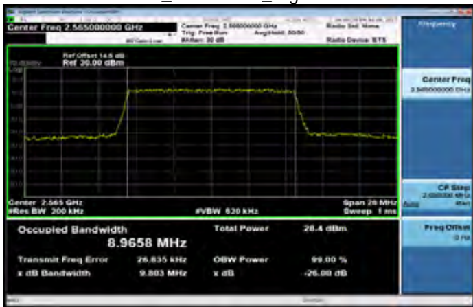
Band7 10MHz_QPSK 50_0_HighCH21400-2565
