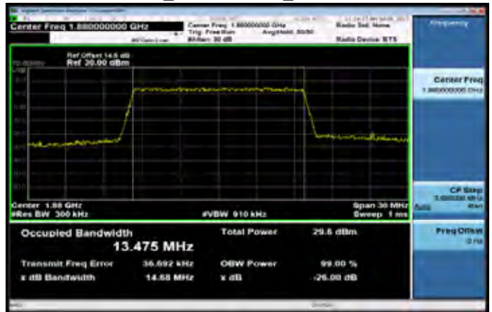
Band2 15MHz_16-QAM 75 0_MidCH18900-1880
