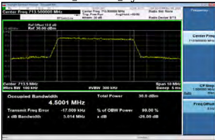
Band12 5MHz_QPSK 25 0_HighCH23155-713.5
