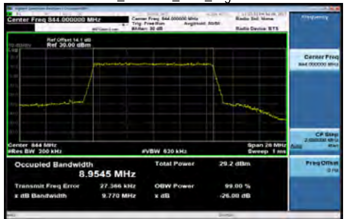
Band26 10MHz_16-QAM_50 0_HighCH26990-844
