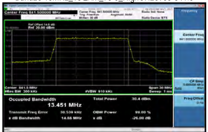
Band26 15MHz_16QAM_75 0_HighCH26965-841.5
