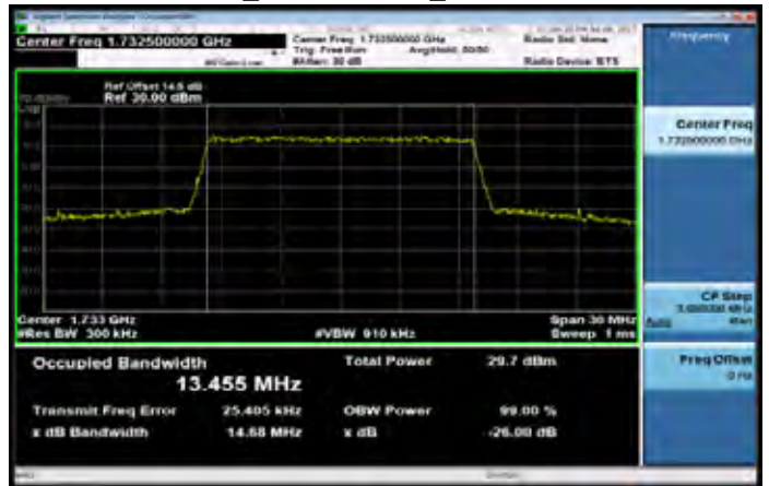
Band4 15MHz_16-QAM 75 0_MidCH20175-1732.5
