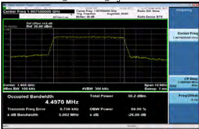
Band2 5MHz_QPSK 25 0_HighCH19175-1907.5
