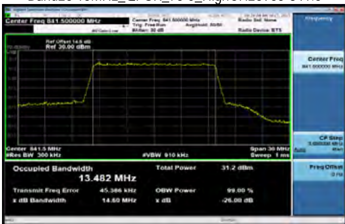
Band26 15MHz_QPSK_75 0_HighCH26965-841.5
