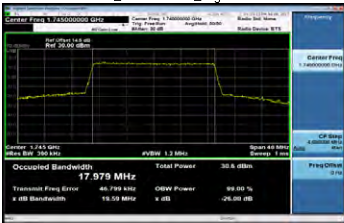
Band4 20MHz_QPSK 100 0_HighCH20300-1745
