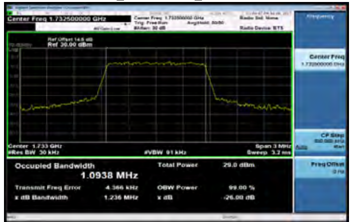
Band4 1.4MHz_16-QAM 6 0_MidCH20175-1732.5
