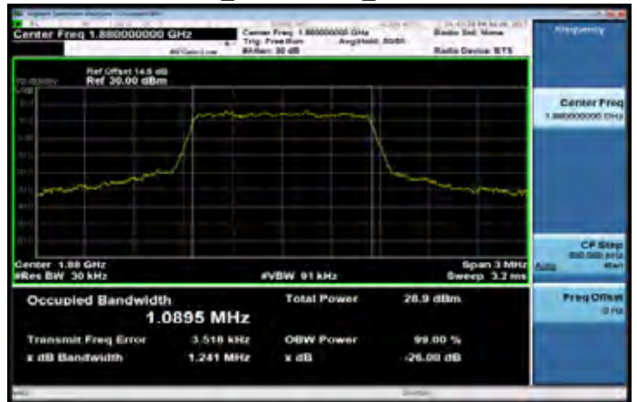
Band2 1.4MHz_16-QAM 6 0_MidCH18900-1880
