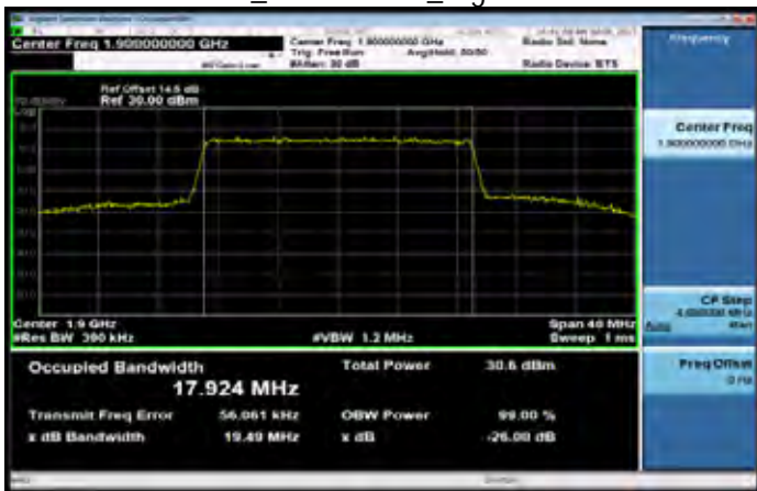
Band2 20MHz_QPSK 100 0_HighCH19100-1900
