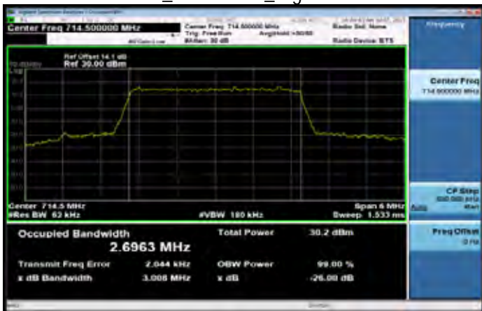
Band12 3MHz_QPSK 15 0_HighCH23165-714.5
