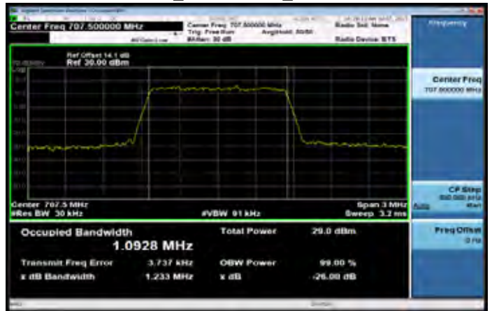
Band12 1.4MHz_16-QAM 6 0_MidCH23095-707.5
