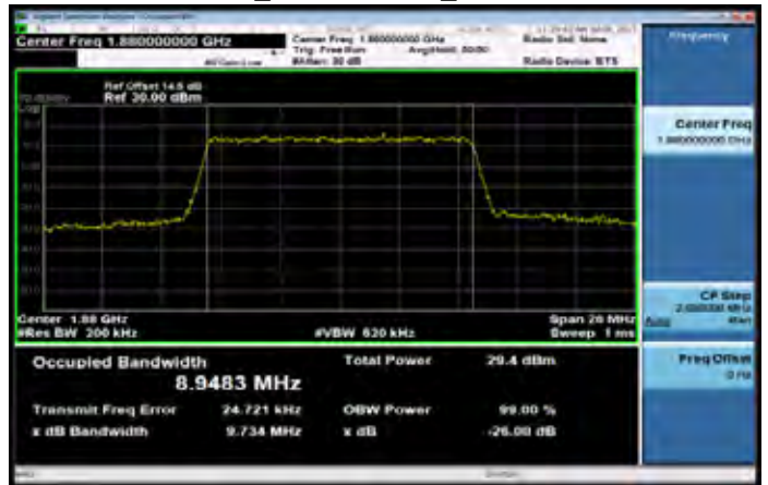
Band2 10MHz_16-QAM 50 0_MidCH18900-1880
