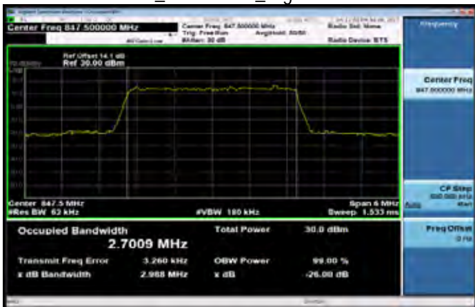
Band5 3MHz_QPSK 15 0_HighCH20635-847.5
