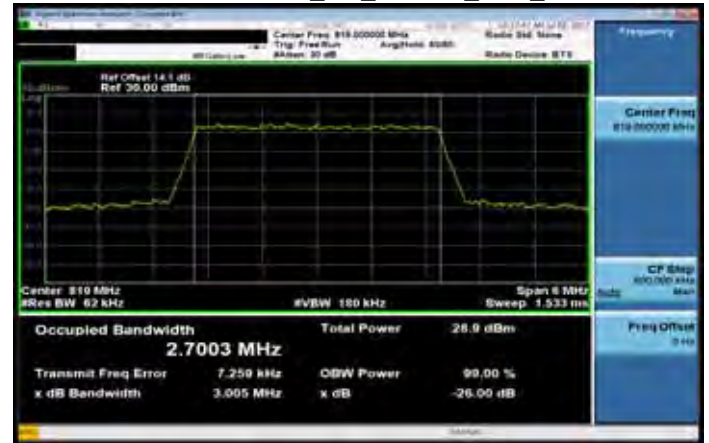
LTE Band 26 for Part 90S_3M_16QAM_15 0_MidCH26740
