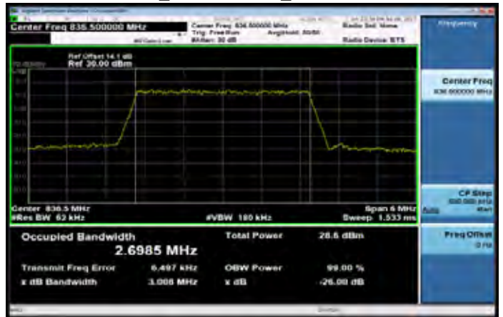
Band5 3MHz_16-QAM 15 0_MidCH20525-836.5
