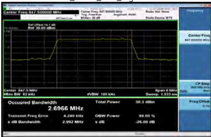
Band26 3MHz_QPSK_15 0_HighCH27025-847.5
