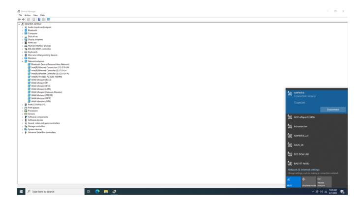
After driver installation, you should see the Intel AC9260 device in the device manager and be able to connect with AP in your space.
