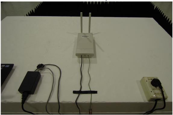
Conducted Setup Photo (Measurement at Antenna Port)
