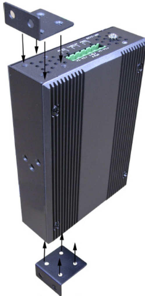
Figure 2.13 Combining the Metal Mounting Kit
