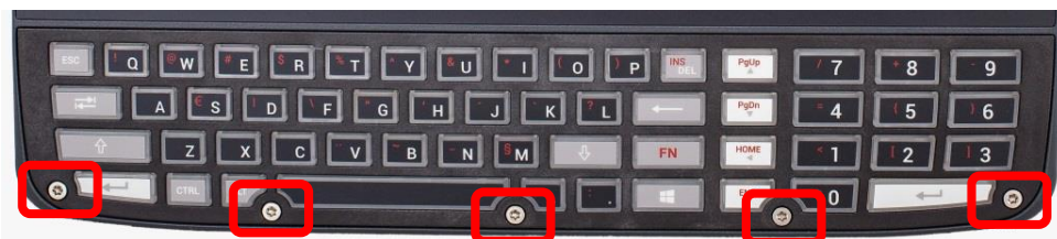
Fig. 16.1: Integrated keyboard: Unscrew the mounting screws
