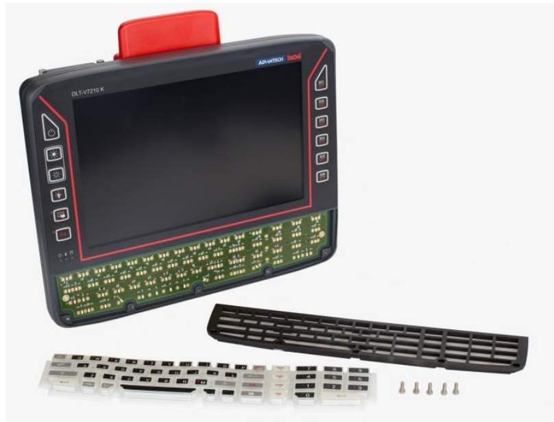
Fig. 16.2: Integrated keyboard: Keyboard components
