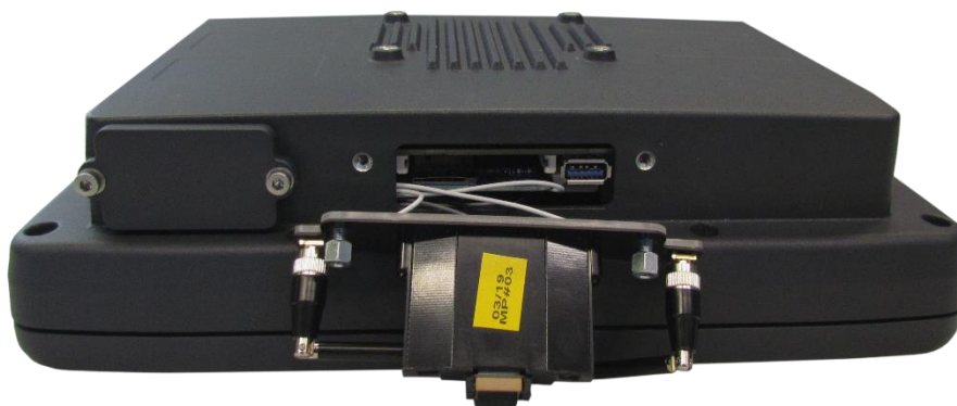
Fig. 7.10: Antenna module WLAN, WWAN LTE 4G is open
