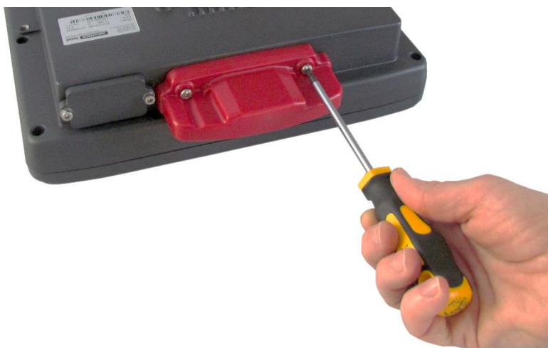
Fig. 7.8: Opening the WLAN, WWAN LTE 4G antenna (Torx Tx20)
