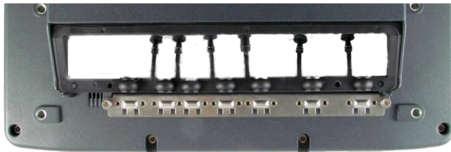
Fig. 13.4: Rubber seal inserted in the cable compartment
