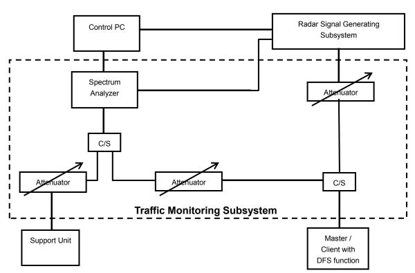
The test transmission will always be from the Master Device to the Client Device. While the Client device is set up to associate with the Master device and play the MPEG file (6 ½ Magic Hours) from Master device, the designated MPEG test file and instructions are located at: <a href="http://ntiacsd.ntia.doc.gov/dfs/">http://ntiacsd.ntia.doc.gov/dfs/</a>.
