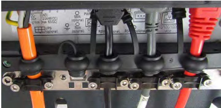
Fig. 12.8: Unused cable outlets sealed off with blind plugs
