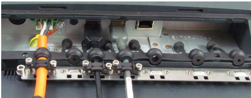
Fig. 12.5: USB cable on the connector panel; secured to the strain relief rail
