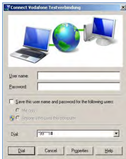
Fig. 10.9: SIERRA WIRELESS MC80 – Dial test connection
