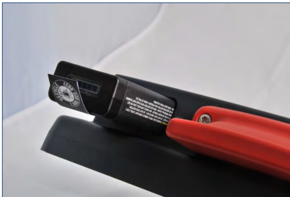
Fig. 15.2: Inserting the battery pack in the battery pocket
