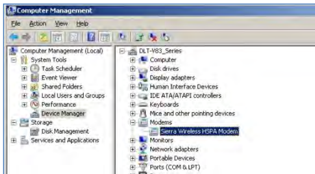
Fig. 10.2: SIERRA WIRELESS MC80 - Device manager, Sierra Wireless HSPA Modem
