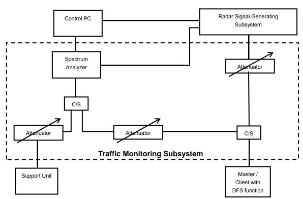
Conducted setup configuration of ADT DFS Measurement System
