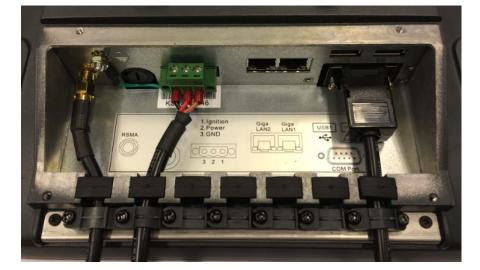
Fig. 6.8: Unused cable outlets sealed off with blind plugs
