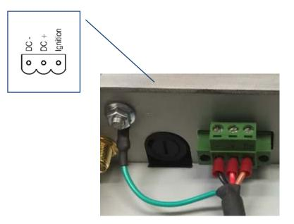
Fig. 8.1: DC power supply connector with power cable connector detail view
