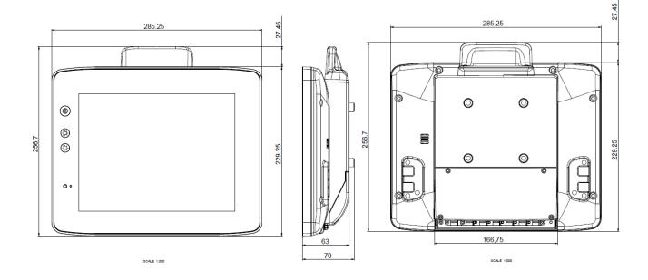
Fig. 11.2: Dimensions of DLT-V6210
