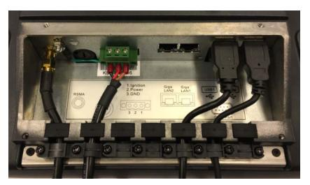
Fig. 6.5: USB cable on the connector panel; secured to the strain relief rail
