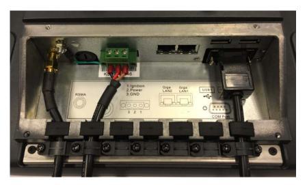
Fig. 6.7: COM cable on the connector panel; secured to the strain relief rail
