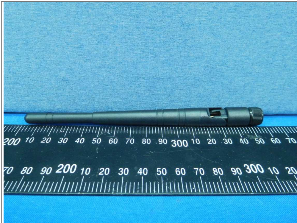
Dipole Antenna (Brand: Taoglas Model: GW.59.3153)
