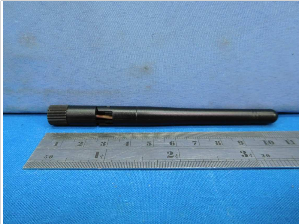
Dipole Antenna (Brand: San Jose Model: UEN-201)
