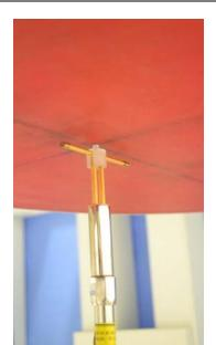
Construction: Symmetrical dipole with I/4 balun Enables measurement of
