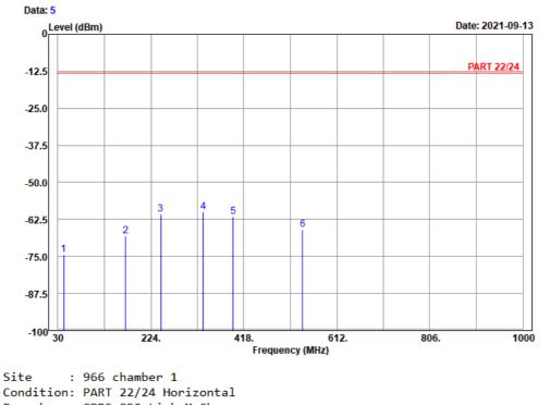
Condition: PART 22/24 Horizontal Remark : GPRS 850\_Link\_M-Ch Tested by: Karl Lee Read Limit Over Freq Level Level Line Limit Factor Remark
