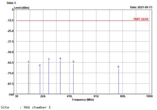
Site : 966 chamber 1 Condition: PART 22/24 Horizontal Remark : GPRS 850\_Link\_M-Ch Tested by: Karl Lee Read Limit Over
