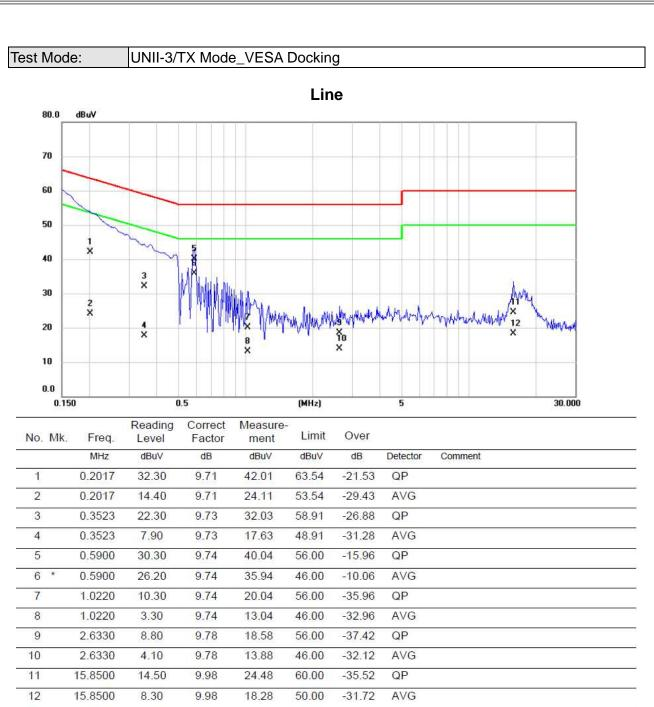
Note : The test result has included the cable loss.
