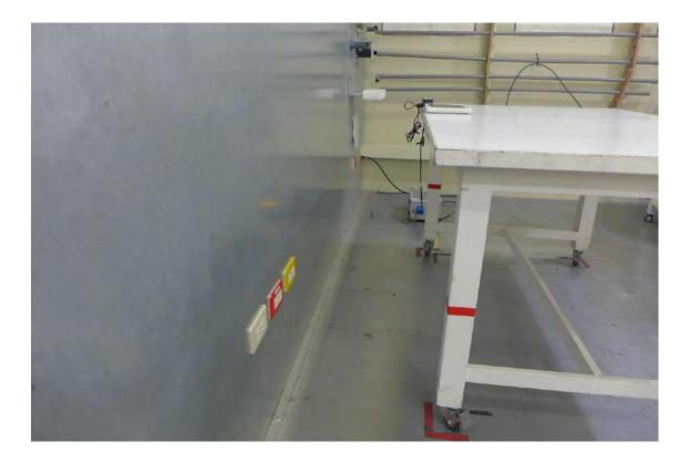
Conducted Measurement Photos Adapter: FSP / FSP065-DBCM1+ VESA Docking
