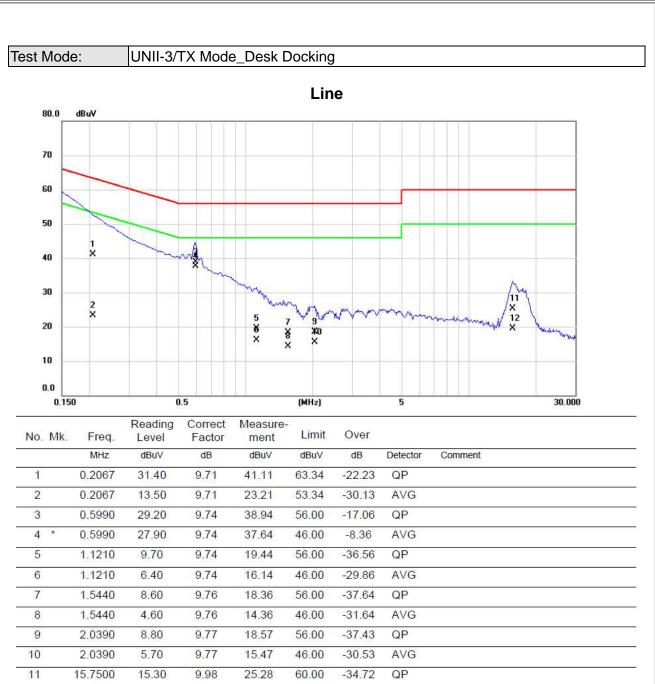
Note : The test result has included the cable loss.
