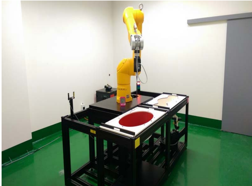
Liquid depth in the flat Phantom ( \geq 15\text{cm} depth) Body(750MHz)_15.6cm Body(835MHz)_15.7cm
