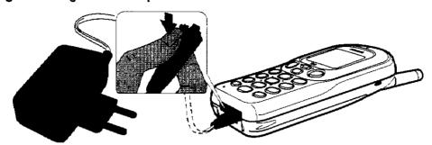
· Plug the transformer unit into a mains AC power socket.
