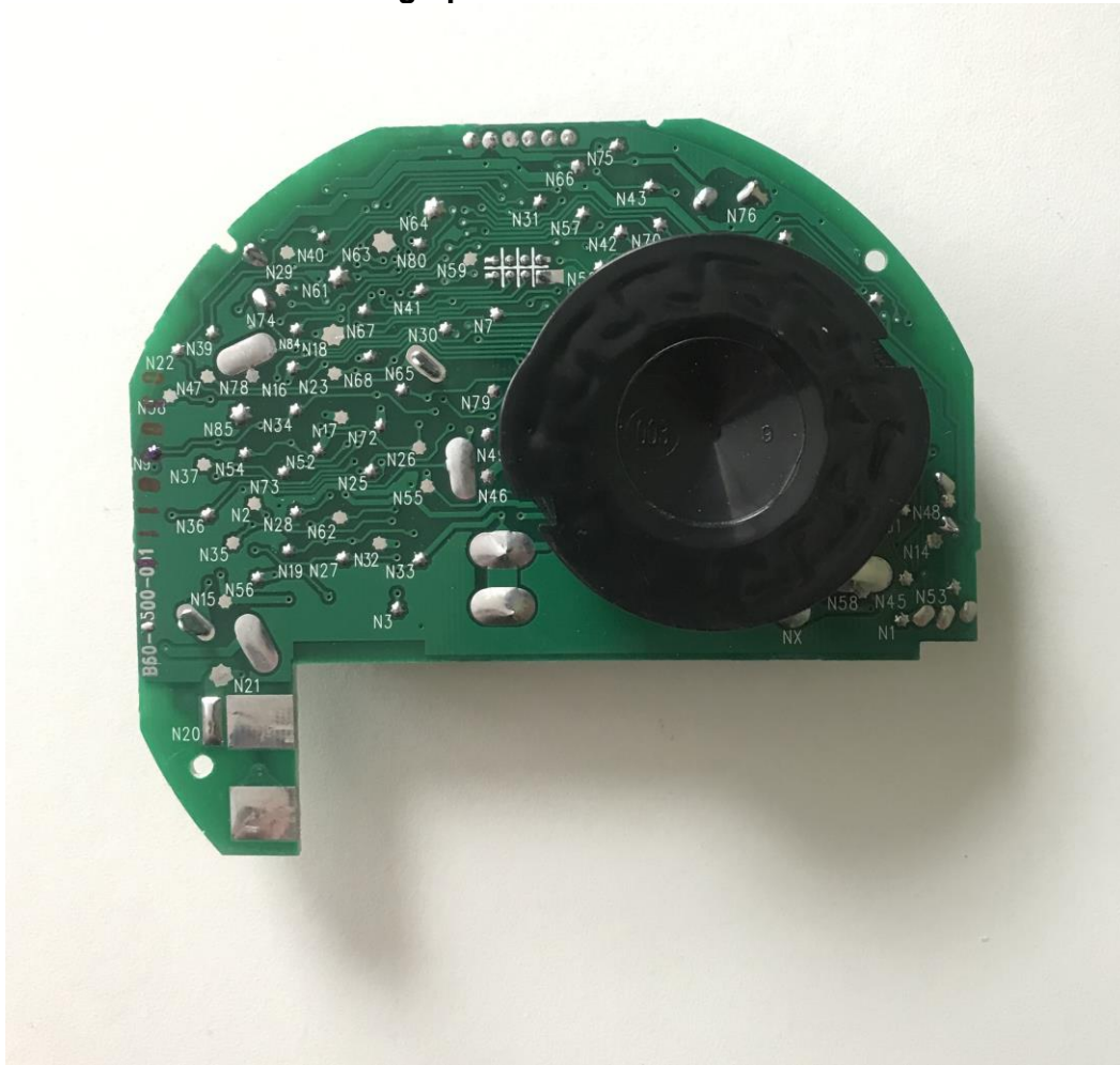
Photograph of PC Board: Foil Side
