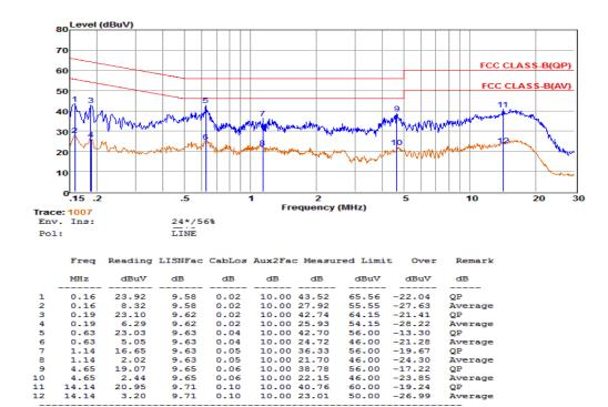
Measured = Reading +Cable Loss +Aux2 Fac.
