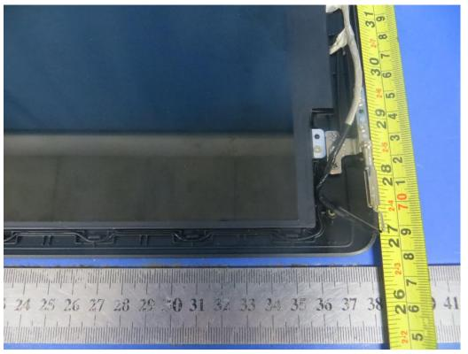
The distance is 210mm of antenna to Bottom of Laptop
