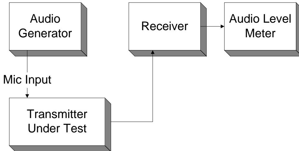
**Para. No. 2.987(b) - Modulation Limiting**
