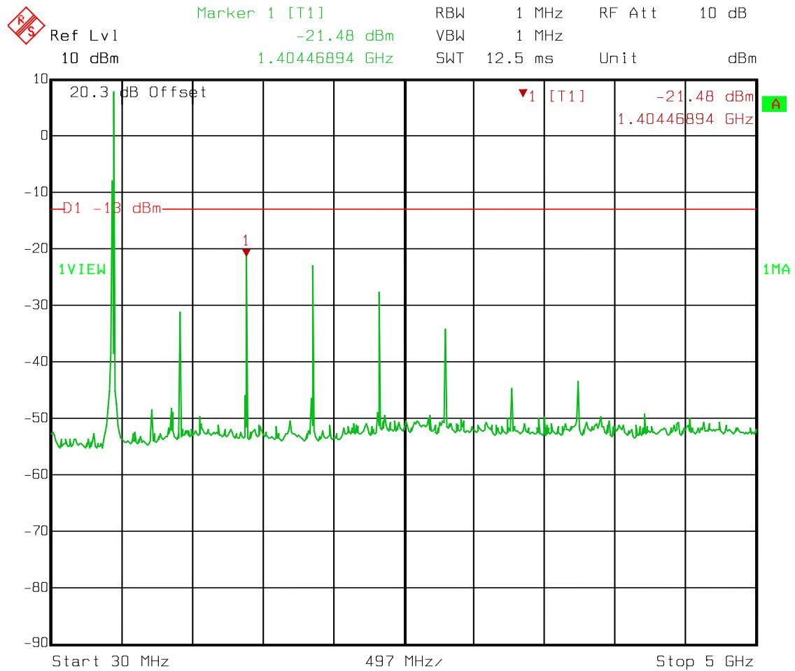
EQUIPMENT: TX-9560PROJECT NO.: 10248775\_TRF\_FCC90-RSS119\_Rev1**Section 6. Field Strength of Spurious Emissions**
