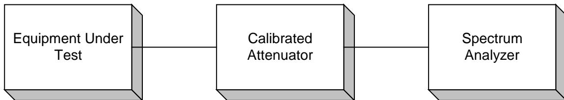
**Para. No. 2.993 - Field Strength of Spurious Radiation**
